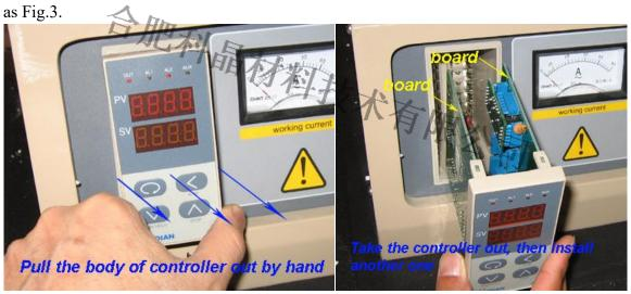
Fig.3 uninstallation of temperature controller, step 2 and step 3
